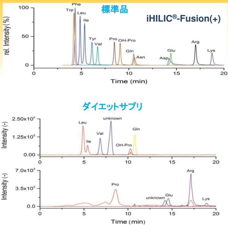
**LC-MS System:** Agilent 1100er LC system and Thermo Fisher LTQ™ equipped with a HESI source, operated in positive ionization mode for analysis of standards. For the dietary supplement, an Orbitrap™ Exactive classic equipped with a HESI source and operated in positive ionization mode.
